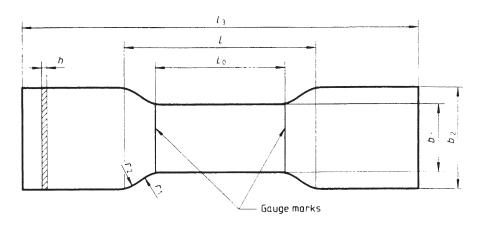
$b_1$  Width of narrow parallel-sided portion: 25,4 mm  $\pm$  0,1 mm
